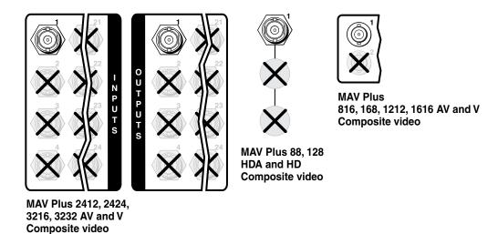
Figure 2-15 — MAV Plus video connections
